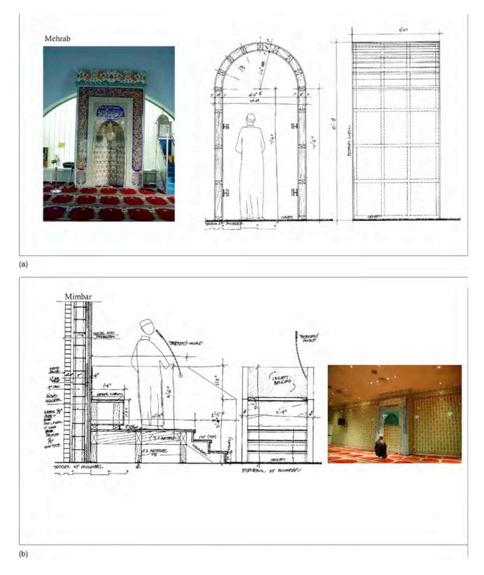
Figure 4.7 (a) Detail of the *mihrab*. (b) Detail of the *mimbar*. (Drawings by Latif Abdulmalik)
